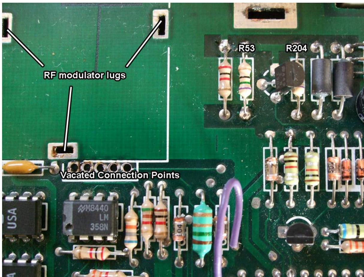
2. With the RF modulator removed, our next job is to replace the resistors R53 and R204 (on either side of the transistor Q3) with 75ohm resistors as shown in the preceding illustration.
