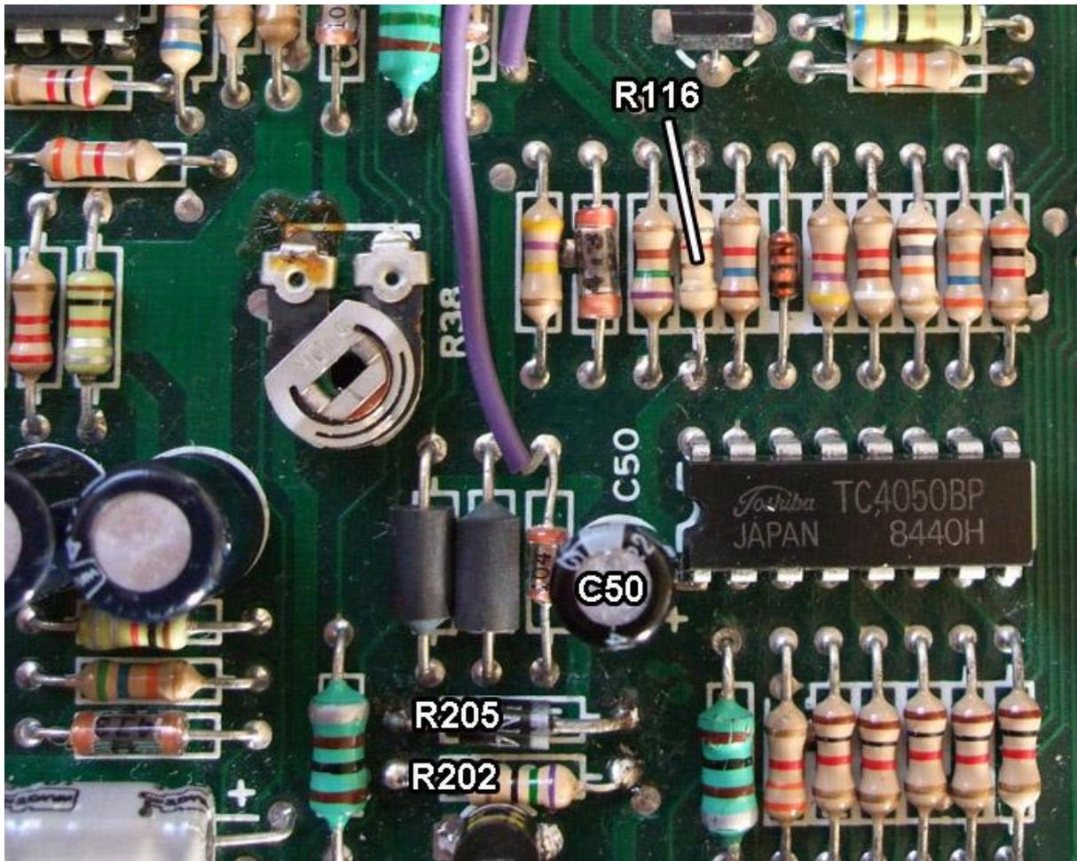
3. Now, moving towards the front of the board (pictured above), we need to replace R116 with an 8.2ohm resistor.
